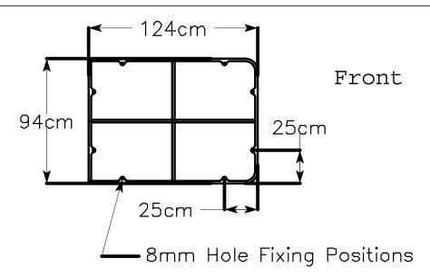
All Steel Construction. Self Build can be Bolted or Welded to this subframe.
